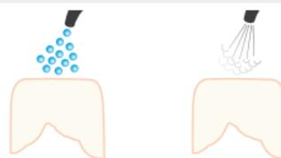
Completely remove any remaining acid by using water spray (60 sec.) or clean in the ultrasonic bath.
